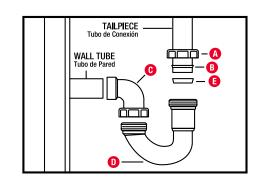
Tighten nuts. CHECK FOR LEAKS.
