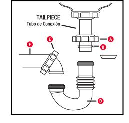
Tighten all nuts. CHECK FOR LEAKS.
