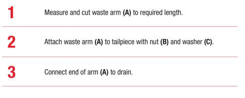
Λ Tighten nuts. CHECK FOR LEAKS.
