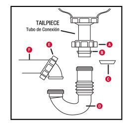
Tighten all nuts. CHECK FOR LEAKS.
