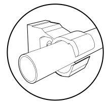
To unlock, simply add pressure and open the clamp.
